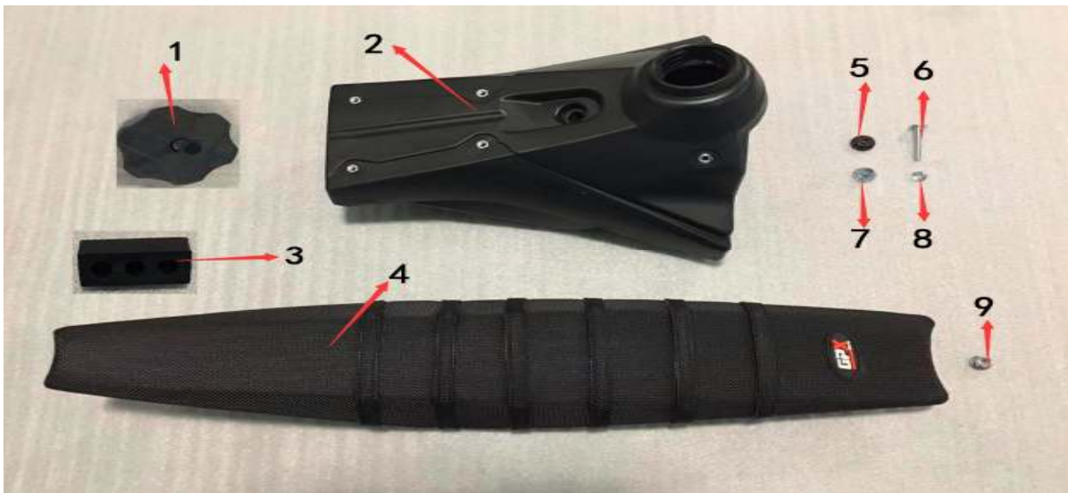
Figure G: the cushion, oil tank, tubing, etc. (图G: 坐垫、油箱组件等)
